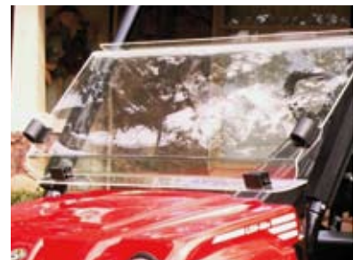
Shatter-resistant windshield that meets AS-5 glazing specifications.
